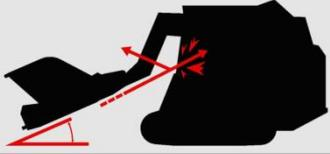
Rotating disc and thrown objects can cause serious injury, death or cause serious machine damage. Be aware of mulcher angle to prevent damage or injury.
